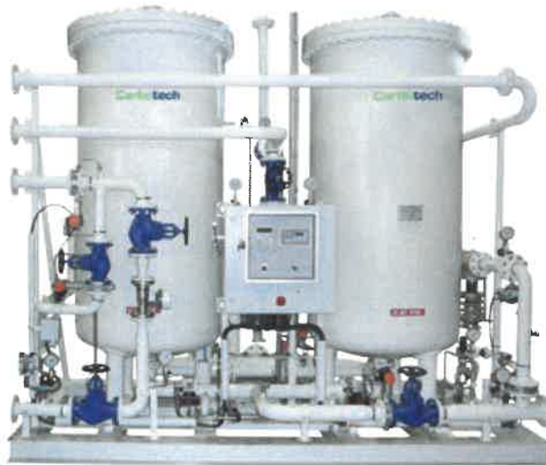
Units for hydrogen, above, and nitrogen generation are designed and built by Carbotech on the basis of individual application requirements.
